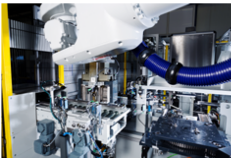
Transfer of the cylinder head from the intake roller conveyor
