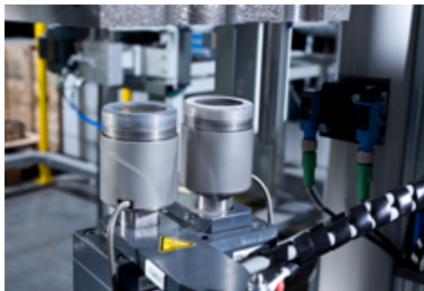
Pressing in of nitrogen-cooled valve seat rings
