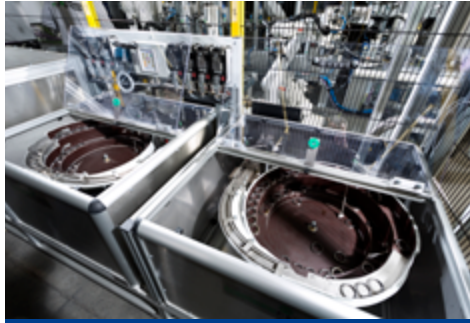
Automatic supply of valve seat rings
