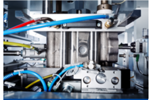
Leak test of oil chamber using the pressure difference procedure
