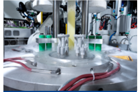
Automatic fitting of the liquid nitrogen tank with valve seat rings and valve guides
