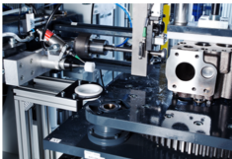
Loctite wetting and pressing in of threaded bushings and closure caps
