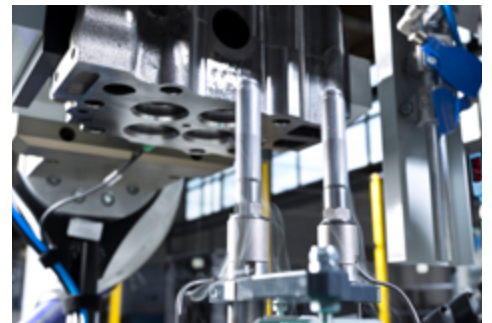
Pressing in of nitrogen-cooled valve guides
