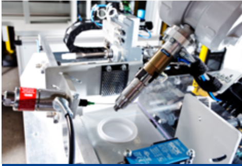
Loctite wetting of injector sleeves
